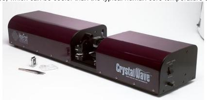
Low thermal mass is needed to reach the temperature setpoint in relatively short amount of time. However, at the same time the temperature change should be sufficiently slow for the IOL material to adjust. The cuvette allows for simple temperature control to ensure proper
