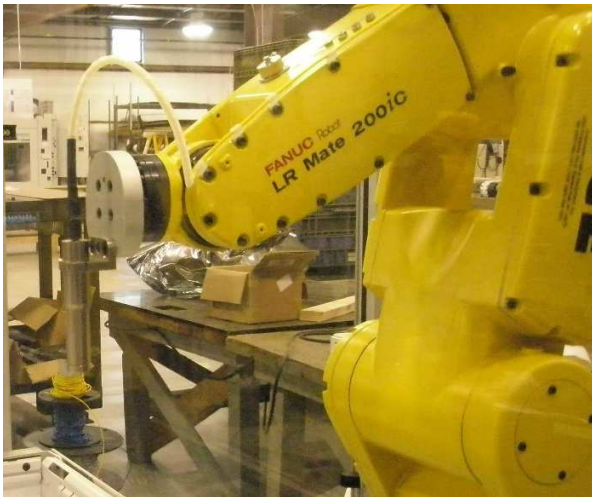
Probe integrated with robot
