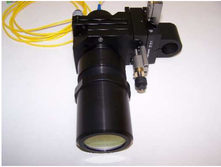
Large diameter 2 foot focal length probe
