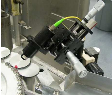
Online testing of ampoule dome thickness
