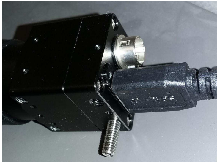
Figure 2: CLAS-FX wavefront sensor USB3 cable installed
