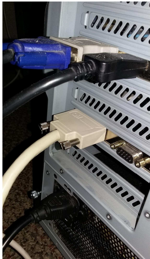
Figure 5: Legacy CameraLink framegrabber installed in computer with white CameraLink communications cable connected
