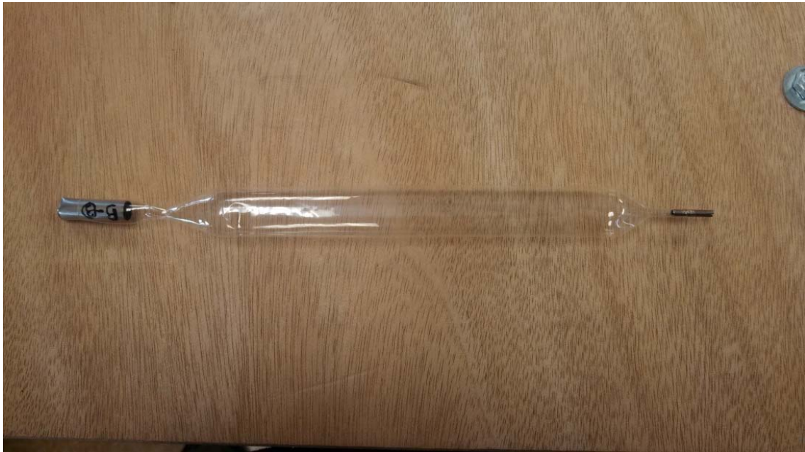
Figure 5 - Sample B with the Small Metal Tubes Installed
