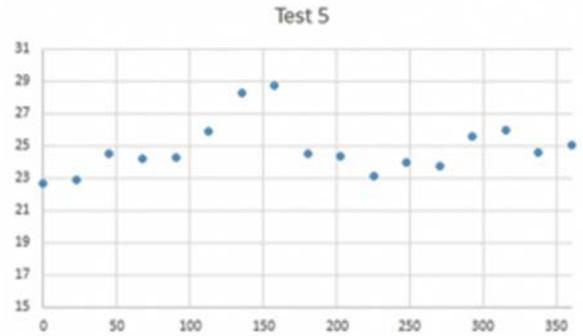
Figure 4 - Balloon wall thickness over 360-degree rotation
