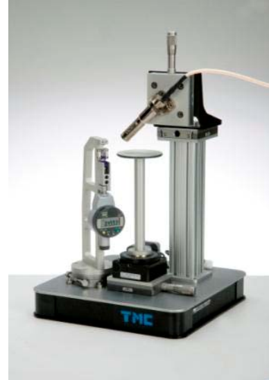
Figure 2: Glass Ampoule Positioning Fixture and OptiGauge Probe Assembly
