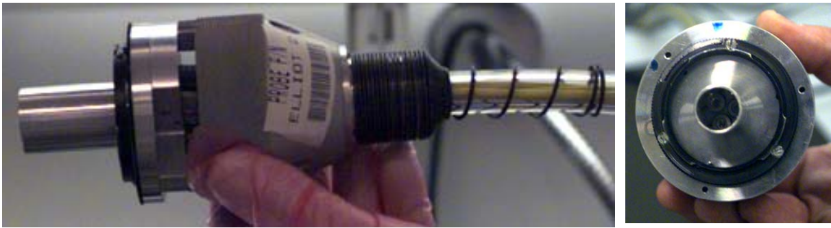
Figure 5. Optical probes for assessing imager focus in Canon EOS (left) and Nikon Pronea-based (right) camera bodies
